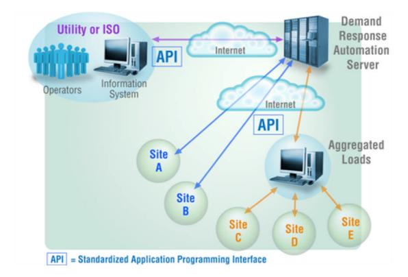
The OpenADR standard specifies the application programming interfaces (APIs) to, and the functions of, the Demand Response Automation Server (DRAS), which serves as the common platform between all providers and consumers of electricity.
