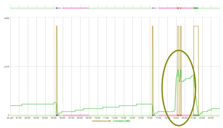
During a shed from 5:00 to 9:00, you can see a large draw (green goes up), and water heater comes on to 'top off'
