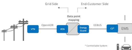
If the communication behind the grid connection fails, the heartbeat mechanism of the EEBUS ensures that the devices operate in a fail-safe mode and return to a normal operation as soon as the communication is re-established. The configurable polling mechanism within OpenADR allows a periodic message exchange between the VEN and VTN
