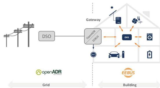
By measuring the power consumption, the DSO may identify hotspots and take in-time corrective action by limiting power consumption via setpoints. In addition to controlling the power demand, the feed-in
