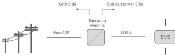
Both, OpenADR and EEBUS use cases are fully specified and already widely in use in the industry. The system delivers high value in end-to-end security, capacity, and tariff management.
