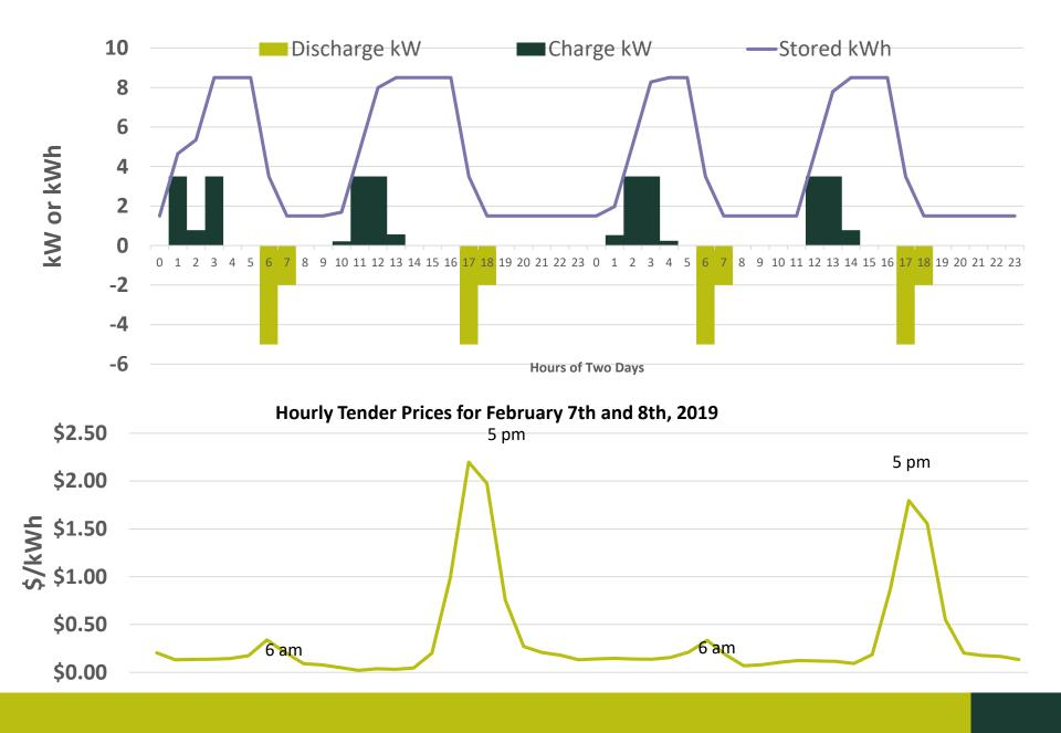
**Operating Results:** 14 kWh / Day Discharge 15.56 kWh / Day Charge
