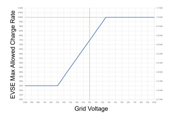
EVSE automatically adjust outputs based on measured grid voltage
