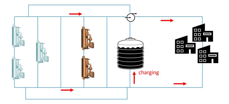
**ADR Event Start:** Chillers automatically turn on and charge thermal storage tank and/or provide campus cooling
