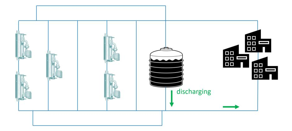
**Afternoon**: Use thermal storage tank to provide chilled water for campus cooling without running chillers
